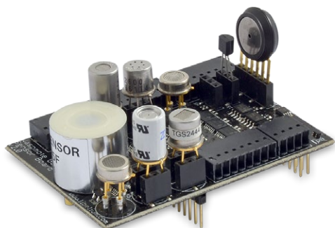
Figure: Gases Board
