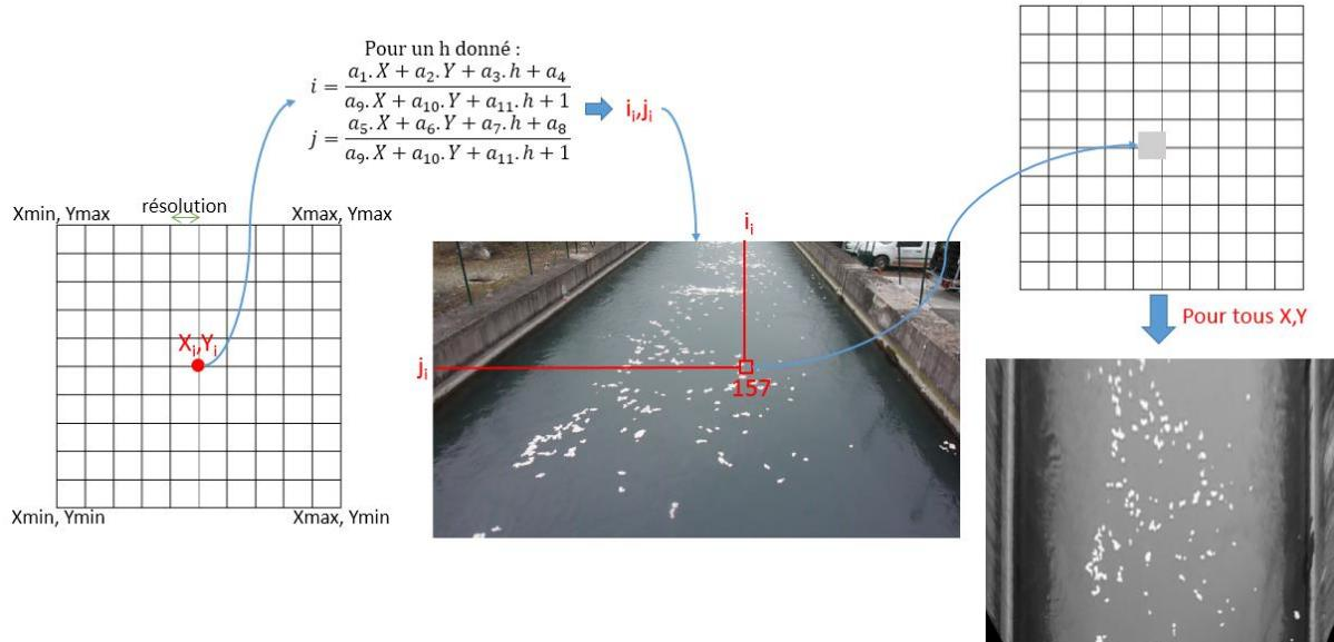
Principles of measuring the velocity of movement of tracers
