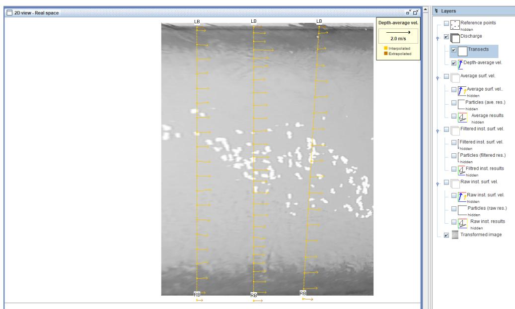
After selecting the transects of interest, the **Discharge → Transect(s) 3D View** menu allows a 3D visualization of the bathymetry of the transects, the height of water and velocities averaged over the depth.
